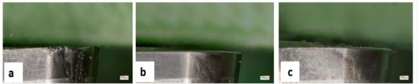
Optical microscope images of tool wear under different conditions; a: Flood, b: SAC without nanoparticle and c: SAC with MnS additive
